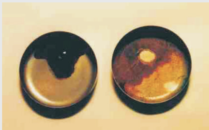
Fig. 3: Residues after storage at 250 °C (482 °F) left: competitors product - right: TURMOFLUID 40 BK
