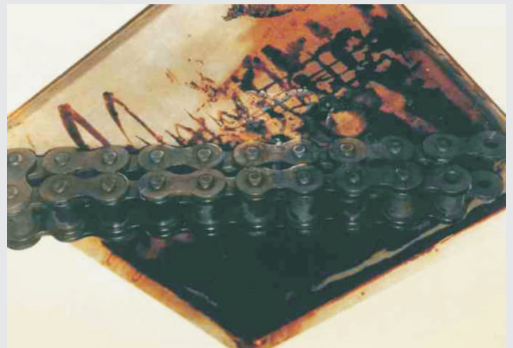
Fig. 2: Roller chain after operation Lubricated with a competitor's product
